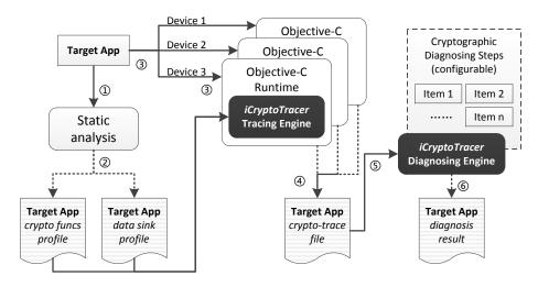
Fig. 6. Overview of *iCryptoTracer* architecture
